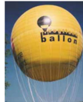
Mylau balloon, 7,5 years of operation without deflation.
